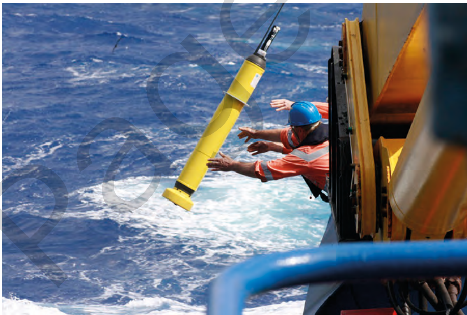
FIGURE 3.3.8 Researchers launch an Argo robotic float from Southern Surveyor . Argo is a collection of 3800 freely drifting floats that measure the temperature, salinity and speed of the ocean. CSIRO and other organisations use data from these floats for climate modelling.
